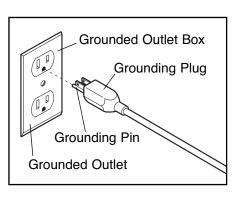
current to reduce the risk of electric shock. This product is equipped with a cord having an equipmentgrounding conductor and a grounding plug. Plug the power cord into an appropriate outlet that is properly installed and grounded in accordance with all local codes and ordinances. This product is for use on a nominal 120-volt circuit. IMPORTANT: The elliptical exerciser is not compatible with GFCI-equipped outlets.
